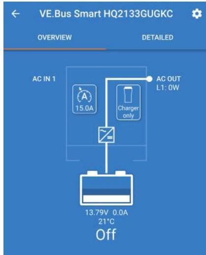
The button on the left will allow you to limit how much amperage you can draw from your shore power source. By default, it will be set to 30A as the trailer uses a 30A inlet plug. However, you may want to change this limit temporarily if you are on a 20A or 15A outlet to prevent tripping the breaker on your power source.
