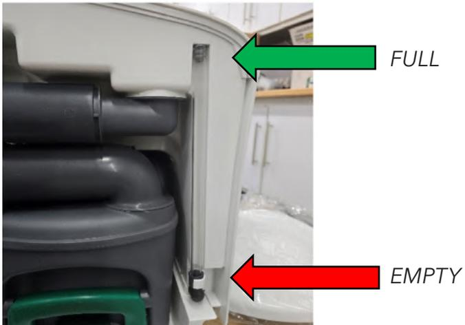
To drain the flush water tank gently pull down on the sight glass tube and swing it outwards to pour the contents of the tank into an appropriate container. Reseat the sight glass and empty the flush water in an appropriate place.
